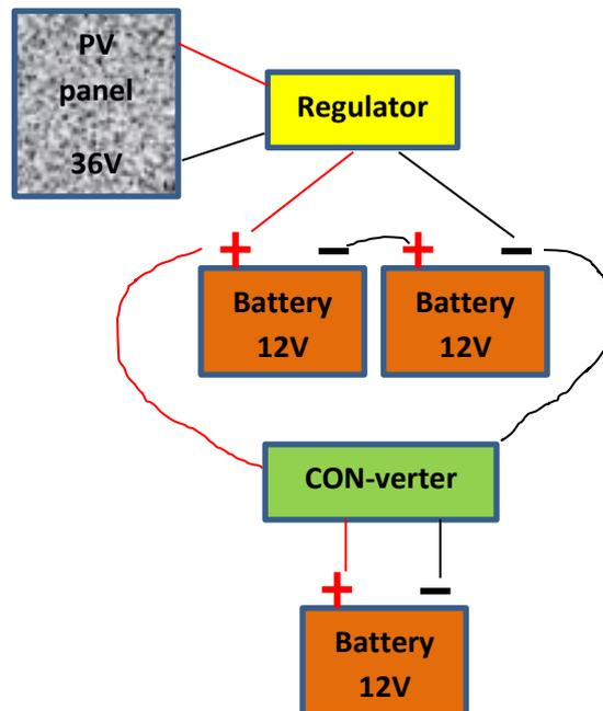
With this layout you charge a 12V battery from a converter. The benefit of this option is that you can exceed the current capacity of the converter during operational cycles, provided there is enough time between cycles to charge the battery.
