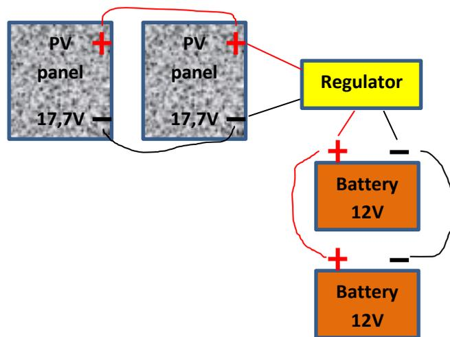
This works fine, as long as your maximum power draw remains below 200W. For larger power draw systems the voltage of the battery bank must be increased to reduce the current draw. Thus for the typical inverter systems, ie computers and tv's, you want a 24V system. Starting from scratch you may use components with the following values :
