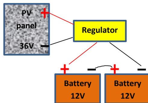
NOTE – see how you connect two batteries in SERIES to obtain a 24V power pack.
