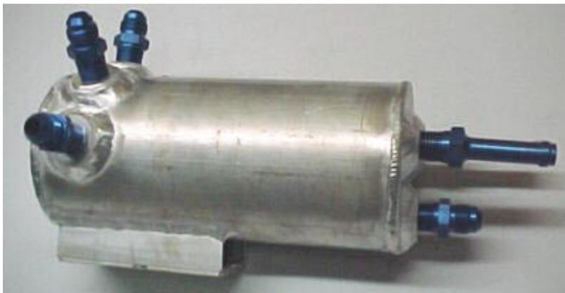
This tank has 3 lower fittings for twin pumps plus a drain fitting. Earls NPT weld-in bosses are used. This tank is made from 3 inch, 6061 T6 tubing. Mild steel exhaust tubing also works well. All joints are carefully TIG welded. Test for leaks before installing.
