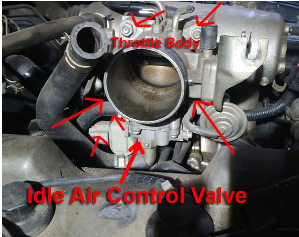
remove throttle body
