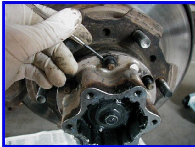
Then again, on my spare axle, which appeared to be totally stock and had never been taken apart, the screwdriver technique didn't work but a quick tap with a hammer on the hub popped off one after another cone washer with ease (several of which flew off with such force, that if I didn't have the nut loosely on the end, I would have lost them as they flew off into the grass).
