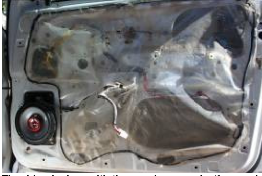
The driver's door with the panel removed – the speaker and plastic sheet clearly visible.
