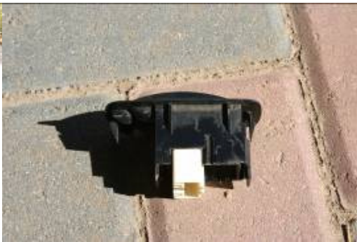
The rear door's window switch – once removed.
