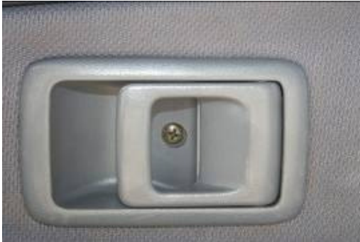
Retaining screw clearly visible
