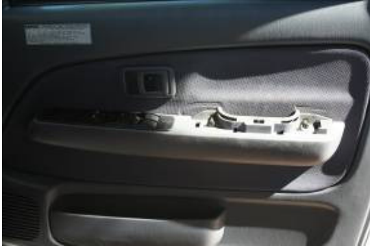
The driver's door panel with the armrest removed to expose the #3 Philips screws (x2) on either side of the "U" shaped area on the right side of the photo.
