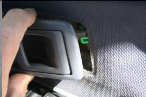
The green retainer between the door release and door panel, clearly visible.
