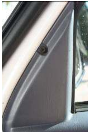
Flathead screw halfway up the triangular piece of the doorpanel.
