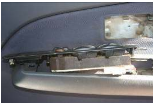
The electric window switch panel once removed.
