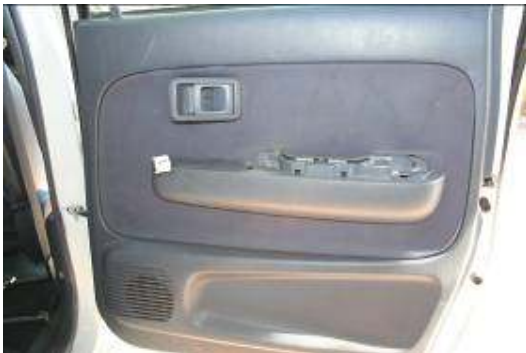
The driver side rear door in the same state – the armrest and the window switch removed.
